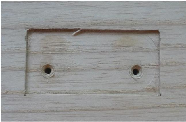
A close-up view of a rectangular hole cut into a light-colored wooden surface. The hole is rectangular with rounded corners and contains two circular holes, one on each side, which are the mounting points for hinges.                                                      |
