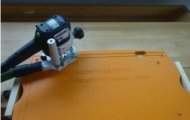
A hand-held router is shown in use on a wooden surface. A yellow template is placed over the work area. The router is a black and green model with a white base. The template has the text 'Kopierdüse 30mm' and 'Werkzeuggestrichmesser 18mm' printed on it. |
