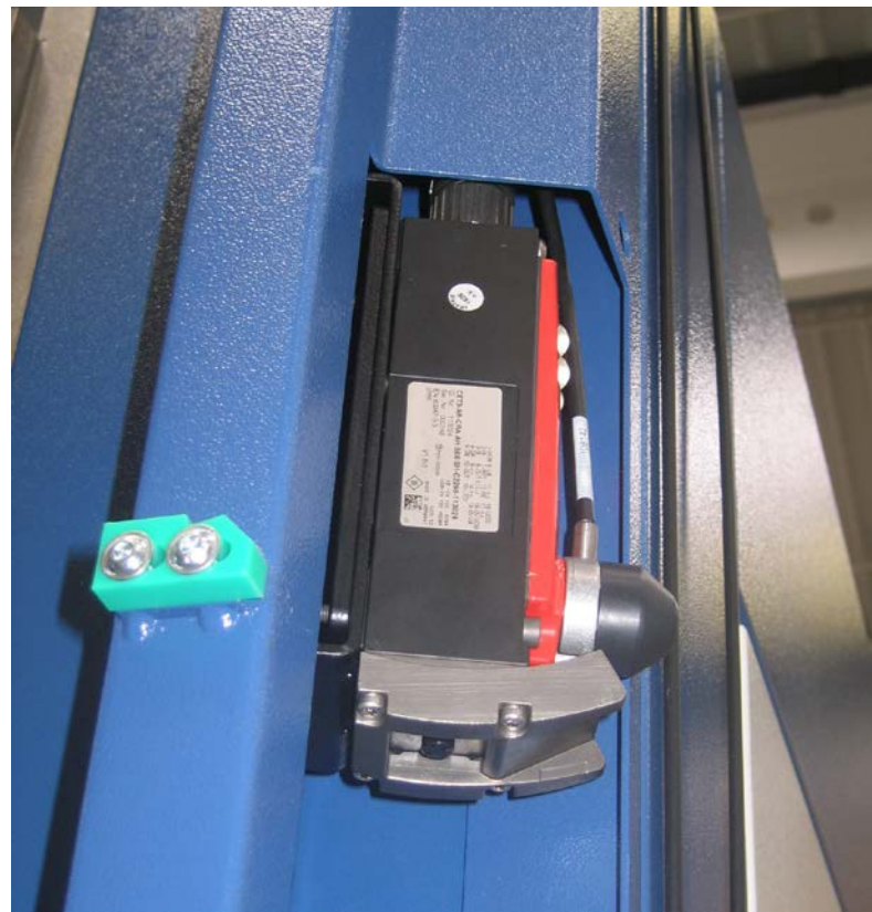
Figure 5 Interlocking guard with guard locking/position switch with emergency unlocking by Bowden cable
